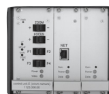
Single-camera rack with video server
